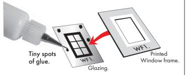
Using a fine tip applicator, place tiny spot of **UHU** glue on the edges of the glazing and then fix the window frame on top.
