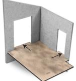
Fit the floor with the two doorway tabs sticking through the door openings. Fixed to the door bottoms.
