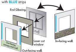
Push out the window opening from the laser cut card sheet L1. Now attach the glazing to the back of it so that the printed glazing sit centrally in the opening. Next fix the laser cut window to the back of the out-facing wall, all edges flush, then fix the in-facing wall to the back of the glazing.
