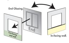
Fit the window unit inside the building with openings centred.
