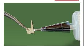
Hold the support with tweezers and very carefully place tiny spots of glue on the back and the base.
