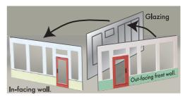
The in-facing and out-facing walls fit together back to back with the glazing sandwiched in between.
