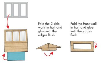
Fold up this position tab (marked above in blue) and glue fast.
