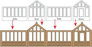
Carefully align the windows to the openings with the matt side of the windows facing through. Glue into place with tiny spots of glue.
