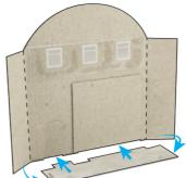
Now add the base, the doorsteps fitting through the doorways, with the inner wall sitting atop the base, the outer wall fitting flush between the spaces between the doorsteps. Wrap the side tabs around and glue flush against the base sides.
