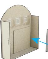
Using the wall support for the correct building (either A,B,F,H or C,D,E,G) Fit tight into the corner, leaving a 1mm recess from the back edge of the side tab and
