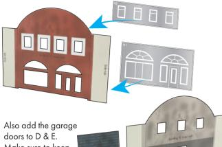
doors to D & E. Make sure to keep the base of the door flush with the bottom edge of the Inner wall.
