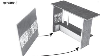
Now add the roof detail. Carefully centre the brown roof section from the sides and keep it flush to the rear.
