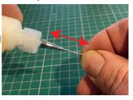
If this doesn't help, then take the metal nozzle off and rod it out with the pin from the other end.
