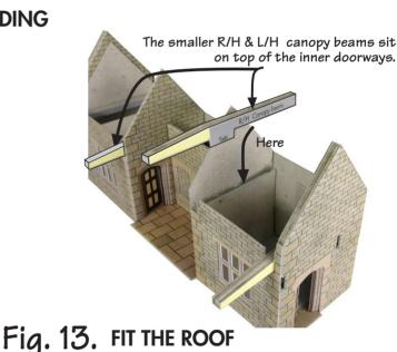
Fitting the roof is self explanatory. But you may find it a little tight against the end walls, in which case you may need to shave a fraction off the end of the roof to make it fit.
